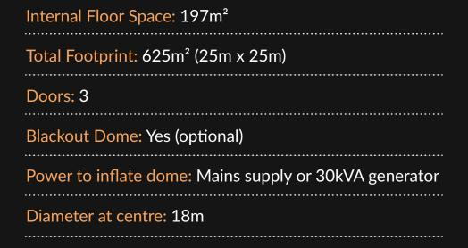
The 18m StratoSphere is an incredibly versatile structure that can be used for a number of different purposes. Its 3-way door alignment makes for easy access and exit and can be installed with either revolve, airlock doors or a combination of the two.
